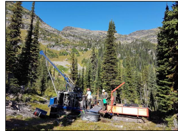
Tracked drill minimizes trails and tree-cutting
